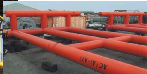
The one-coat glass flake reinforced polyester coating which can be applied by airless spray to achieve a dry film thickness of 30 - 40 mils in a single coat.
