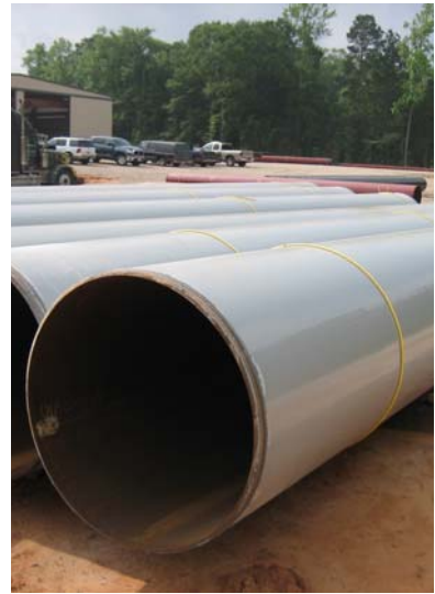
Pipe coated with 30 mils of Protal 7900HT.
